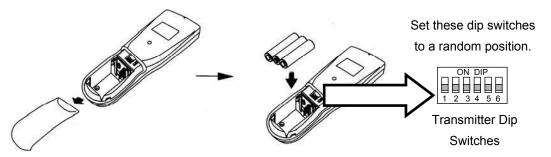
3 Position the transmitter within 1 foot of the receiver. The LED indicator panel on the transmitter should be flashing (if not, remove and replace the batteries). Press down any button on the transmitter until the receiver "beeps". This indicates the transmitter and receiver are calibrated on the same radio frequency (if it does not, unplug receiver, remove batteries, plug in receiver, replace batteries, and repeat this process). Test operation of the remote control.
