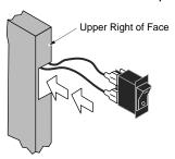
Remove the knob and nut from the rheostat. Insert the shaft on the rheostat through the circular hole on the control panel and secure with the nut. Replace the knob.
