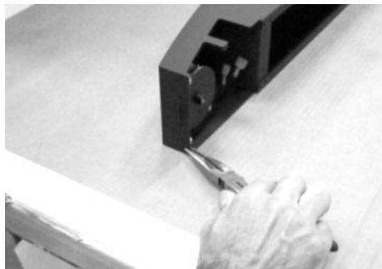
Figure 13: Bending the tab on the face
