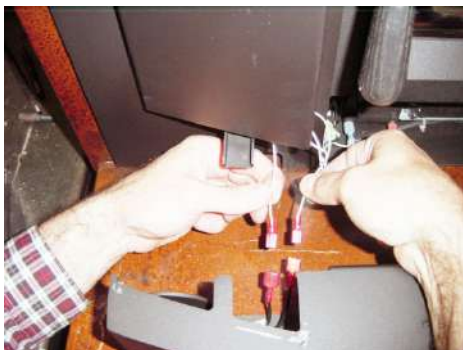
Figure 15: Connecting the bottom left wires
