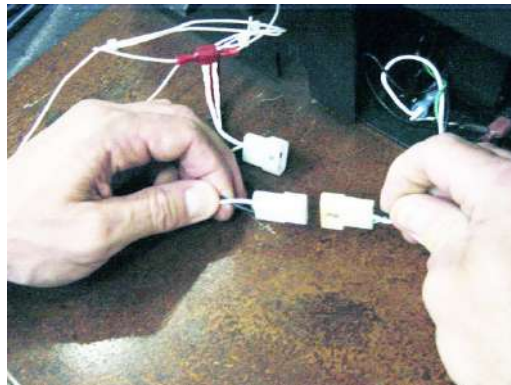
Figure 10: Connecting the Molex connectors
