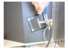
Connect the igniter wires. Orientation of the wires does not matter. Wrap the wires around the compressor hose.
