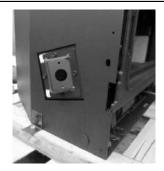
Attach the igniter assembly to the housing using the screws provided, as shown below. Note that the igniter gasket is placed between the housing and igniter assembly.
