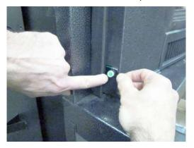
Connect the igniter assembly wires; orientation does not matter. Connect the start button wires to the igniter assembly.
