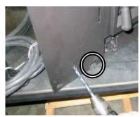
Route the igniter cord through the "mouse hole" in the left side of the panel as shown above. Attach the face to the panel.
