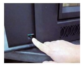
**NOTE:** If you need to turn off the igniter after starting the ignition process, press the GreenStart button a second time. The system will turn off power to the igniter and the GreenStart button will flash. The pump will continue to run for about seven minutes and then shut off.
