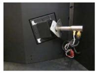
Connect the compressor hose to the igniter as shown and secure with the included hose clamp.
