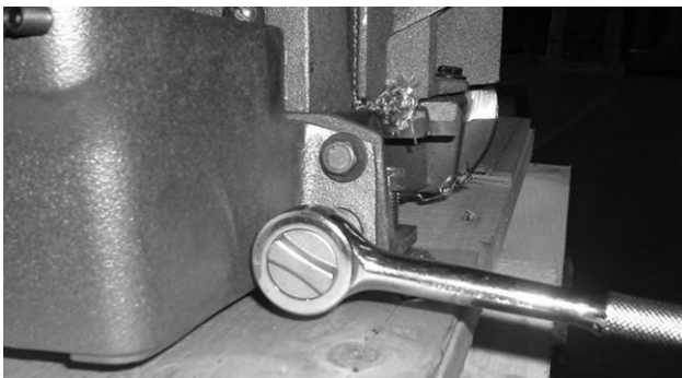
Photo 27 – Ash Lip Assembly Fastener Detail
