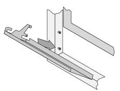
Hold the grill at an angle and insert the lower slot over the bushing on the fireplace (both sides). You may need press on the grill to get the tab over the bushing (this prevents the grill from accidentally falling off).
