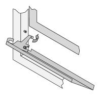
Bend this the tab over on both sides. This is the end-stop for the lower grill, it allows the grill to swing forward.
