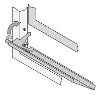
Swing the grill upwards to engage the upper slot. You will need to lift the grill slightly to get it over the bushing. Once in place the grill is held in place by gravity.
